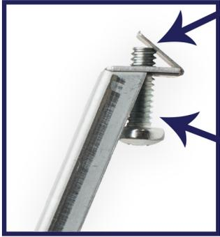
**BINDING TAB:** PREVENTS THE BOLT FROM “WALKING” ON THE SINK RIM. AS THE WEIGHT OF THE SINK PASSES DOWNWARD, IT ALSO CREATES PRESSURE AGAINST THE BOLT, “LOCKING” IT IN PLACE.
